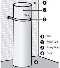
The minimum clearance from the water tank to combustible surface must be 500mm.
