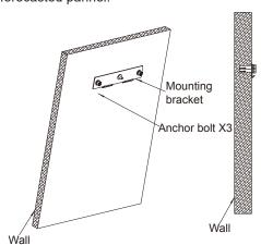
Step3: Attaching indoor unit to the wall.
